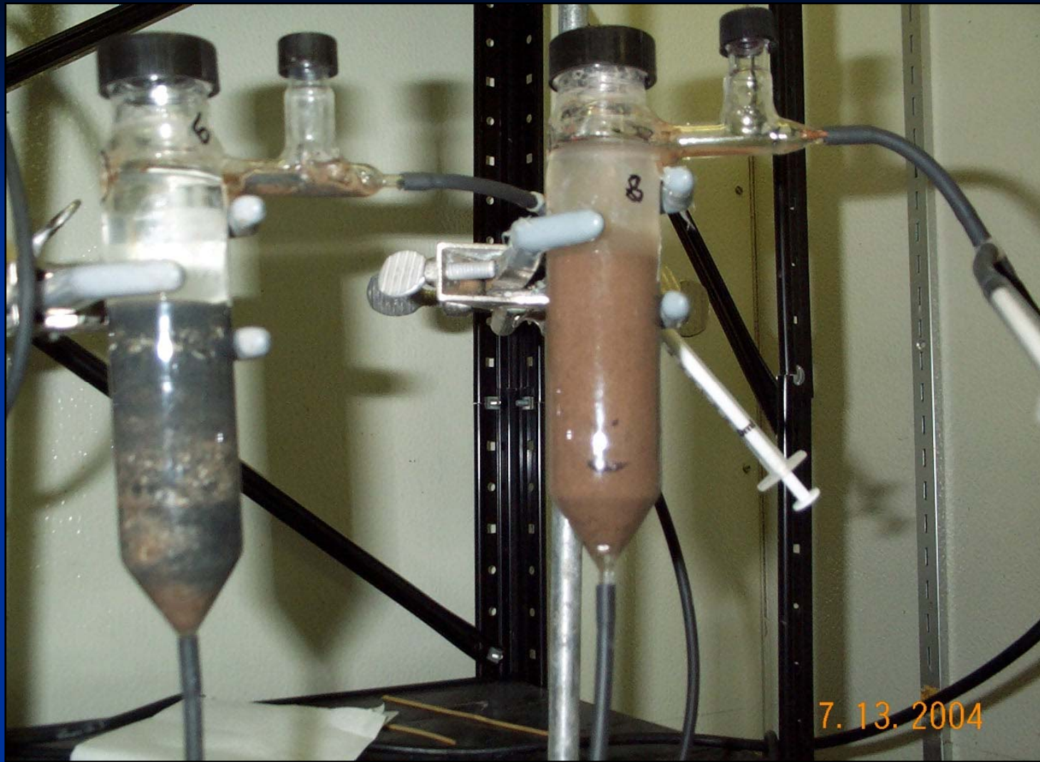
Soil columns with and without Apatite II (Ap) infused with TNT-contaminated groundwater
